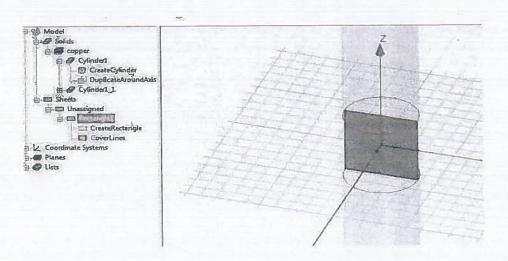
g. Select the drawn rectangle and define it as the input signal area/port HFSS > Excitations > Assign > Lumped Port.
