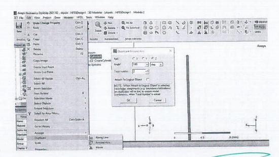
e. Select the first cylinder and then select Edit > Duplicate > Around Axis, choose the axis X or Y and enter the angle of 180°, Total number 2.
